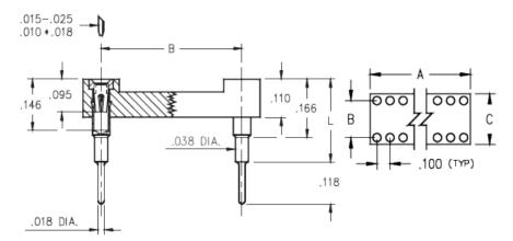
**Description:** DIP Dual In Line Socket Elevated Profile Open Frame Through Hole Plating Code: 93 Shell Plating: 200 μ" Tin/Lead(93/7) over 100 μ" Nickel
