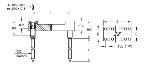
**Description:** DIP Dual In Line Socket Wire-Wrap Tail Open Frame **Plating Code:** Shell Plating: 200 μ" Tin (matte finish) over 100 µ" Nickel Inner Contact Plating: Gold Flash Packaging: Packaged in Tubes
