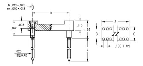
**Description:** DIP Dual In Line Socket Wire-Wrap Tail Open Frame **Plating Code:** Shell Plating: 200 μ" Tin (matte finish) over 100 μ" Nickel Inner Contact Plating: Gold Flash Packaging: Packaged in Tubes
