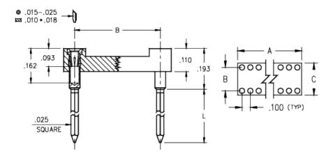
**Description:** DIP Dual In Line Socket Wire-Wrap Tail Open Frame **Plating Code: Shell Plating:** 200 μ" Tin/Lead(93/7) over 100 μ" Nickel **Inner Contact Plating:** 30 μ" Gold over 50 μ" Nickel Packaging: Packaged in Tubes
