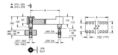
**Description:** DIP Dual In Line Socket Solderless Press-Fit Open Frame Through Hole Plating Code: 43 Shell Plating: 200 μ" Tin (matte finish) over 100 u" Nickel Inner Contact Plating:
