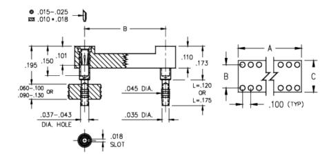
**Description:** DIP Dual In Line Socket Solderless Press-Fit Open Frame Through Hole Plating Code: 43 Shell Plating: 200 μ" Tin (matte finish) over 100 u" Nickel
