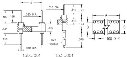
**Description:** DIP Dual In Line Header Solder Tail DIP Header .025" (0,64mm) Pin Head
