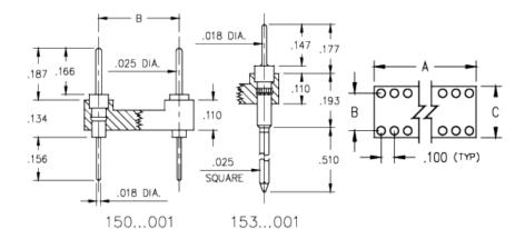
**Description:** DIP Dual In Line Header Solder Tail DIP Header .025" (0,64mm) Pin Head Open Frame Through Hole Plating Code:
