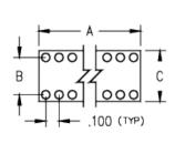
**Description:** DIP Dual In Line Socket Standard Solder Tail Closed Frame Through Hole Plating Code: 13 **Shell Plating:** 10 μ" Gold over 100 μ" Nickel **Inner Contact Plating:**
