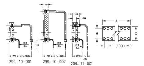
**Description:** DIP Dual In Line Socket Right Angle Mount Closed Frame Through Hole Plating Code:
