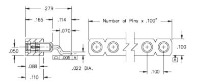
Interconnect Socket Horizontal Mount Socket Accepts .015"- .025" (0,38 - 0,635 mm) dia leads Single Row Surface Mount **Plating Code:** 43 Shell Plating: 200 µ" Tin (matte finish) over 100 µ" Nickel Inner Contact Plating: 30 µ" Gold over 50 µ" Nickel
