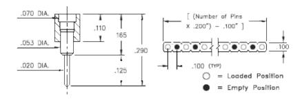
**Description:** Interconnect Socket Standard Solder Tail Socket Accepts .015"- .025" (0,38 - 0,635 mm) dia leads Single Row Through Hole Plating Code: **Shell Plating:** 200 μ" Tin (matte finish) over 100 μ" Nickel **Inner Contact Plating:**
