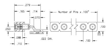
Interconnect Socket Horizontal Mount Socket Accepts .015"- .025" (0,38 - 0,635 mm) dia leads Single Row Surface Mount **Plating Code:** 43 Shell Plating: 200 µ" Tin (matte finish) over 100 µ" Nickel Inner Contact Plating:
