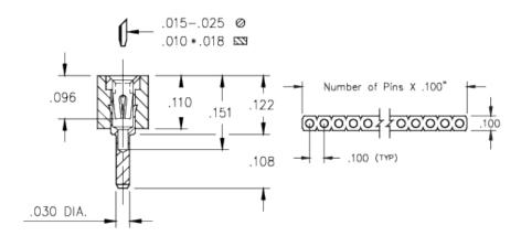
**Description:** Interconnect Socket Low Profile Solder Tail Socket Accepts .015" - .025" (0,38 - 0,635 mm) dia leads Single Row Through Hole Plating Code:
