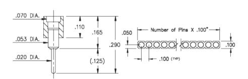
Interconnect Flat Face Target Connector Spring-Loaded Header Vertical Mount Through Hole Target Single Row Through Hole Plating Code: 10 Shell Plating: 10 µ" Gold over 100 µ" Nickel Packaging:
