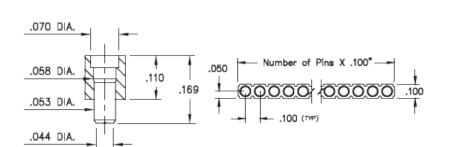
**Description:** Interconnect Target Connector Spring-Loaded Header Vertical Mount SMT Target Single Row Surface Mount **Plating Code:** 10 Shell Plating: 10 µ" Gold over 100 µ" Nickel
