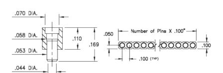
Interconnect Flat Face Target Connector Spring-Loaded Header Vertical Mount SMT Target Single Row Surface Mount **Plating Code:** 10 **Shell Plating:** 10 µ" Gold over 100 µ" Nickel **Packaging:** Packaged in Bulk
