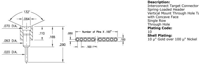
Spring-Loaded Header Vertical Mount Through Hole Target with Concave Face Plating Code: Shell Plating:
