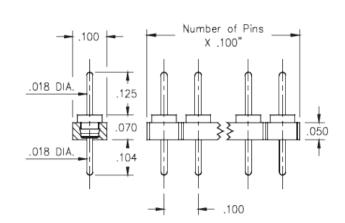
**Description:** Interconnect Header Low Profile Solder Tail Header .018" (0,46mm) Pin Head Single Row Through Hole Plating Code: 10 Shell Plating: 10  $\mu$ " Gold over 100  $\mu$ " Nickel
