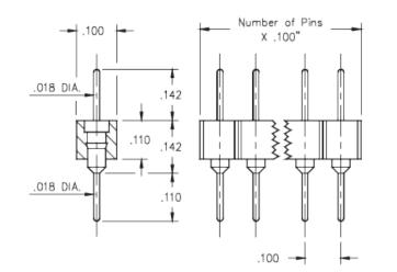
**Description:** Interconnect Header Solder Tail Pin Header .018" (0,46mm) Pin Head Single Row Through Hole Plating Code: 10 Shell Plating: 10 µ" Gold over 100 µ" Nickel
