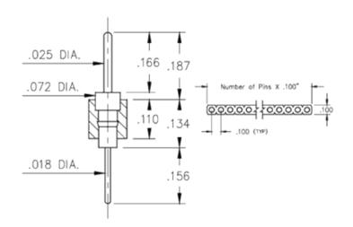
**Description:** Interconnect Header Solder Tail Pin Header .025" (0,64mm) Pin Head Single Row Through Hole **Plating Code:** 10 **Shell Plating:** 10 µ" Gold over 100 µ" Nickel
