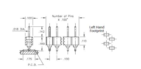
Description: Interconnect Header Surface Mount Pin Header .018" (0,46mm) Pin Head Single Row Surface Mount Plating Code: 10 Shell Plating: 10 μ" Gold over 100 μ" Nickel
