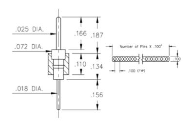
**Description:** Interconnect Header Solder Tail Pin Header .025" (0,64mm) Pin Head Single Row Through Hole Plating Code: 90 Shell Plating: 200 μ" Tin/Lead(93/7) over 100 μ" Nickel
