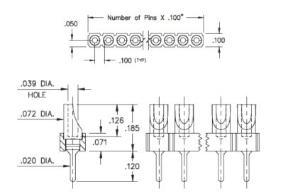
**Description:** Interconnect Header Solder Tail Pin Header SolderCup Head Single Row Through Hole Plating Code: 10 Shell Plating: 10  $\mu$ " Gold over 100  $\mu$ " Nickel
