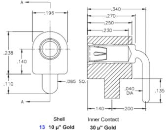
**Description:** Test Point Socket 1.5 mm Black **Plating Code:** Shell Plating:  $10~\mu$ " Gold over  $100~\mu$ " Nickel Inner Contact Plating: 30 μ" Gold over 50 μ" Nickel
