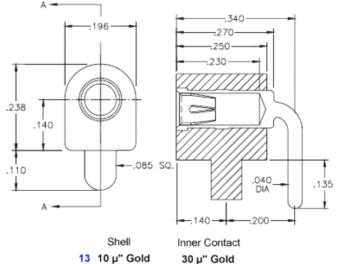
**Description:** Test Point Socket 2.0 mm Black **Plating Code:** Shell Plating:  $10~\mu$ " Gold over  $100~\mu$ " Nickel Inner Contact Plating: 30 μ" Gold over 50 μ" Nickel
