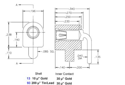
**Description:** Test Point Socket 1.5 mm Black **Plating Code:** 93 Shell Plating: 200 μ" Tin/Lead(93/7) over 100 μ" Nickel **Inner Contact Plating:** 30 µ" Gold over 50 µ" Nickel
