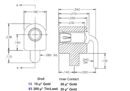
Description: Test Point Socket 2.0 mm Black **Plating Code:** 93 Shell Plating: 200 μ" Tin/Lead(93/7) over 100 μ" Nickel **Inner Contact Plating:** 30 µ" Gold over 50 µ" Nickel
