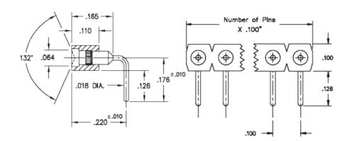
**Description:** Interconnect Concave Face Target Connector Spring-Loaded Header Right Angle Mount Target with Concave Face Single Row Through Hole Plating Code: 10 Shell Plating: 10 µ" Gold over 100 µ" Nickel Packaging: Packaged in Bulk
