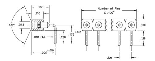
Description: Interconnect Concave Face Target Connector Spring-Loaded Header Right Angle Mount Target with Concave Face Single Row Through Hole Plating Code: 10 Shell Plating: 10 μ" Gold over 100 μ" Nickel Packaging: Packaged in Bulk
