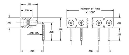
**Description:** Interconnect Flat Face Target Connector Spring-Loaded Header Right Angle Mount Target Single Row Through Hole Plating Code: 10
