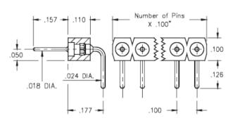
Description: Interconnect Header Right Angle Pin Header .018" (0,46mm) Pin Head Single Row Through Hole Plating Code: 10 Shell Plating: 10 µ" Gold over 100 µ" Nickel
