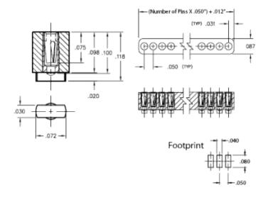
**Description:** Interconnect Socket Surface Mount Socket Accepts .015" - .022" (0,38 - 0,559 mm) dia leads Single Row Surface Mount **Plating Code: Shell Plating:** 200 μ" Tin (matte finish) over 100 μ" Nickel Inner Contact Plating: 10 μ" Gold over 50 μ" Nickel
