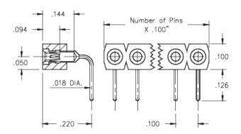
**Description:** Interconnect Socket Right Angle Socket Accepts .015" - .025" (0,38 - 0,635 mm) dia leads Single Row Through Hole Plating Code: **Shell Plating:**
