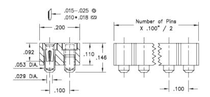
**Description:** Interconnect Socket Surface Mount Socket Accepts .015" - .025" (0,38 - 0,635 mm) dia leads Double Row Surface Mount **Plating Code: Shell Plating:** 200 μ" Tin (matte finish) over 100 μ" Nickel Inner Contact Plating:
