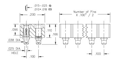
**Description:** Interconnect Socket Surface Mount Socket Accepts .015" - .025" (0,38 - 0,635 mm) dia leads Double Row Surface Mount Plating Code: **Shell Plating:** 200 μ" Tin (matte finish) over 100
