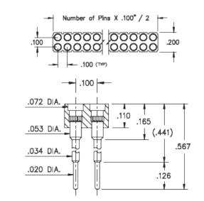
Description: Interconnect Target Connector Spring-Loaded Header Vertical Mount Through Hole Target Double Row Through Hole Plating Code: 10 Shell Plating: 10 µ" Gold over 100 µ" Nickel
