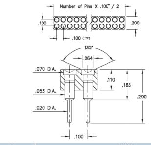
Description: Interconnect Concave Face Target Connector Spring-Loaded Header Vertical Mount Through Hole Target with Concave Face Double Row Through Hole Plating Code: 10 Shell Plating: 10 μ" Gold over 100 μ" Nickel Packaging: Packaged in Bulk
