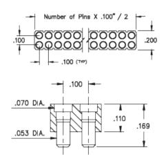
**Description:** Interconnect Flat Face Target Connector Spring-Loaded Header Vertical Mount SMT Target Double Row Surface Mount **Plating Code:** 10 Shell Plating: 10 µ" Gold over 100 µ" Nickel Packaging: Packaged in Bulk
