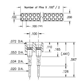
**Description:** Interconnect Flat Face Target Connector Spring-Loaded Header Vertical Mount Through Hole Target Double Row Through Hole Plating Code: 10 Shell Plating: 10 µ" Gold over 100 µ" Nickel Packaging: Packaged in Bulk
