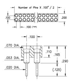
**Description:** Interconnect Flat Face Target Connector Spring-Loaded Header Vertical Mount Through Hole Target Double Row Through Hole Plating Code: Shell Plating:
