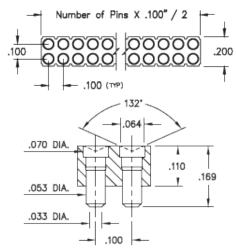
Description: Interconnect Concave Face Target Connector Spring-Loaded Header Vertical Mount SMT Target with Concave Face Double Row Surface Mount Plating Code: 10 Shell Plating: 10 µ" Gold over 100 µ" Nickel Packaging: Packaged in Bulk
