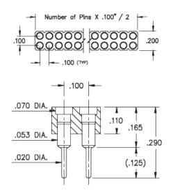
**Description:** Interconnect Flat Face Target Connector Spring-Loaded Header Vertical Mount Through Hole Target Double Row Through Hole Plating Code: 10 Shell Plating: 10 µ" Gold over 100 µ" Nickel Packaging: Packaged in Bulk
