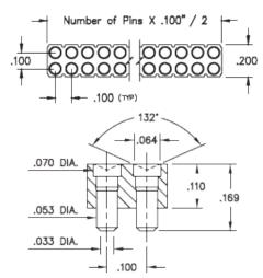
**Description:** Interconnect Target Connector Spring-Loaded Header Vertical Mount SMT Target with Concave Face Double Row Surface Mount Plating Code: 10
