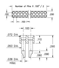
**Description:** Interconnect Flat Face Target Connector Spring-Loaded Header Vertical Mount Soldercup Target Double Row Through Hole Plating Code: 10 Shell Plating: 10 µ" Gold over 100 µ" Nickel Packaging: Packaged in Bulk
