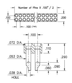
Description: Interconnect Target Connector Spring-Loaded Header Vertical Mount Soldercup Target Double Row Through Hole Plating Code: 10 Shell Plating: 10 µ" Gold over 100 µ" Nickel
