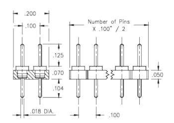
Description: Interconnect Header Low Profile Solder Tail Header .018" (0,46mm) Pin Head Double Row Through Hole Plating Code: 10 Shell Plating: 10  $\mu$ " Gold over 100  $\mu$ " Nickel
