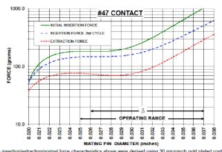
ertion/extraction/normal force cha racteristics above were derived using 30 microinch gold plated contact and polished steel gauge pins having a bullet-shaped tip.
