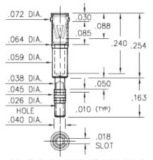
4615-0-31-XX-47-XX-04-0 Compliant press-fit in .040±.003 plated hole. For .090→.130 thick board.
