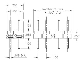
**Description:** Interconnect Header Low Profile Solder Tail Header .018" (0,46mm) Pin Head Double Row Through Hole Plating Code: 10 Shell Plating: 10 µ" Gold over 100 µ" Nickel
