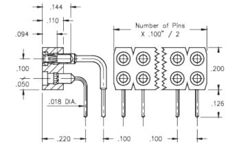
**Description:** Interconnect Socket Right Angle Socket Accepts .015"- .025" (0,38 - 0,635 mm) dia leads Double Row Through Hole Plating Code: 13 Shell Plating: 10  $\mu$ " Gold over 100  $\mu$ " Nickel
